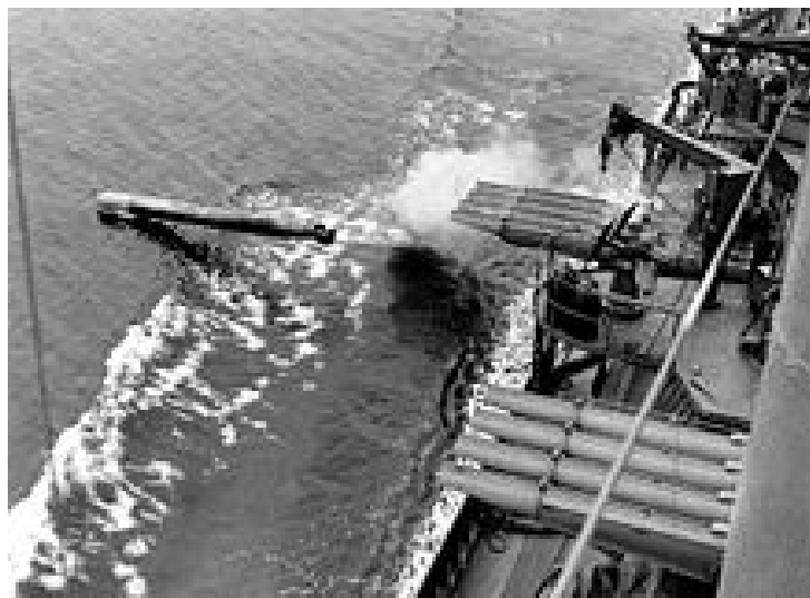
A single MK 15 torpedo being launched from a 4 tube mount during an attack drill. Specifications: 24 ft in length, weight 2,840 lbs., diameter 21 inches. Max. Range/Speed: 6,000 yards at 45 knots Guidance System: Gyroscope Warhead: 825 lbs of explosives
